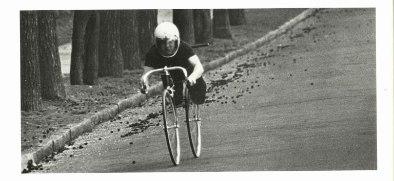
Although radical in its design, the SAE buggy has been a formidable opponent for its four wheel competitors. SAE's "Maroon," designed by Bill Faircloth, takes advantage of bicycle aerodynamics as well as the abilities of an energetic push team.
